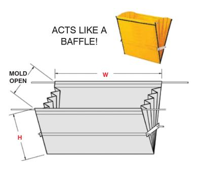
Delayed drops have metal side plates sewn into sides to keep sides rigid.
